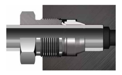
HOKE® is focused on bringing leading edge solutions to the marketplace today. One example is the Integral GYROLOK® feature which eliminates leak paths created by NPT connections and provides a high quality seal that can withstand the severest of application requirements.
