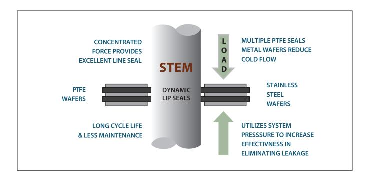
Dyna-Pak<sup>®</sup> provides superior sealing performance while reducing maintenance costs. Consisting of alternate wafers of PTFE and metal spacers, stem leakage is virtually eliminated while the problems associated with PTFE cold flow are minimized.
