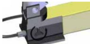
1.3. Remove the protective plug from the inlet connector on the Pre-Setting head, turn counter-clockwise. Keep the plug in a safe place, such as in the black case.
