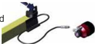
1.2. Open the release valve on hand pump by turning the handle counter-clockwise.
